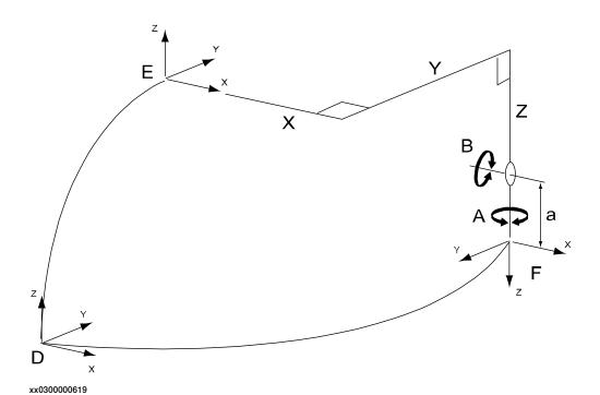
D World frame Ε Base frame F Tool frame Χ X-linear motion Υ Y-linear motion Z Z-linear motion В B rotating around X axis in base frame Α A rotating around Z axis in base frame if B is zero offset\_z of arm
