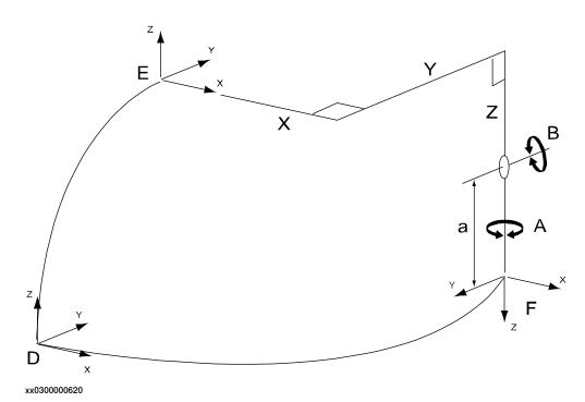
D World frame Ε Base frame F **Tool frame** Χ X-linear motion Υ Y-linear motion Z Z-linear motion В B rotating around Y axis in base frame Α A rotating around Z axis in base frame if B is zero offset\_z of arm
