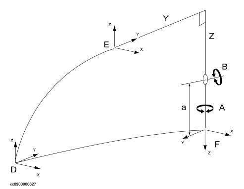
D World frame Ε Base frame F Tool frame Υ Y-linear motion Z Z-linear motion В B rotating around Y axis in base frame Α A rotating around Z axis in base frame if B is zero offset\_z of arm а
